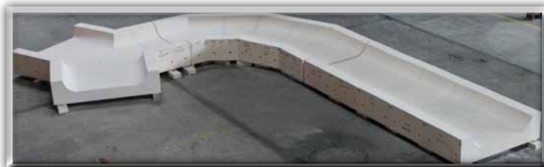
pre-assembly of a feeder channel in a vibro-cast zirconmullite
